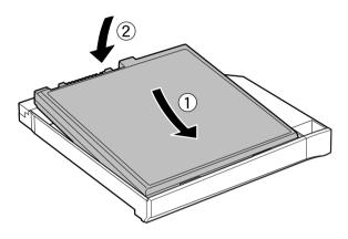
Figure 8-19 Inserting the secondary battery pack in the adaptor
